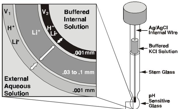
FIGURE 2 pH Glass Electrode Details
